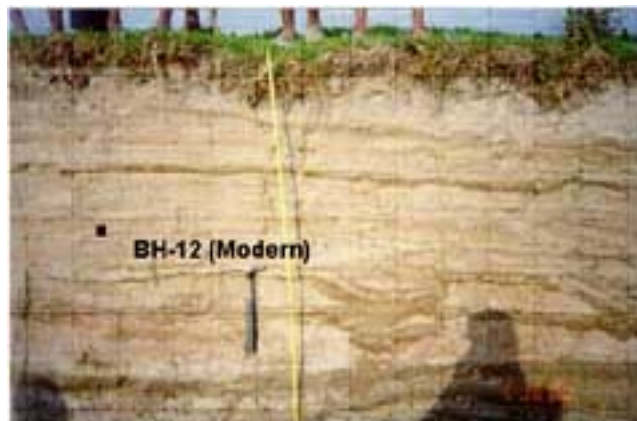
Figure 5. Photograph showing the flexured and disrupted silty sand strata at a depth of 0.7 m subsequent deposition over the disturbed beds had a similar alternating depositional succession as below it. Flexured and disrupted strata is an indication of seismic shaking. The sample BH-12 ( 14 C date ‘Modern’) represents the upper bound for the seismic event (possibly 1934), however the lower bound for this event is lacking.
